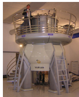
Figure: 900MHz, 21.2 T NMR Magnet at HWB-NMR, Birmingham, UK; credit: wikipedia
